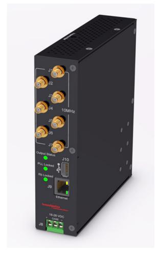
Brandywine's RFS-700D is a miniaturized Rubidium Frequency Reference in a compact ruggedized package designed for mounting on a DIN rail system. The RFS-700D is capable of outputting 7x 10MHz frequency reference with low phase noise.
